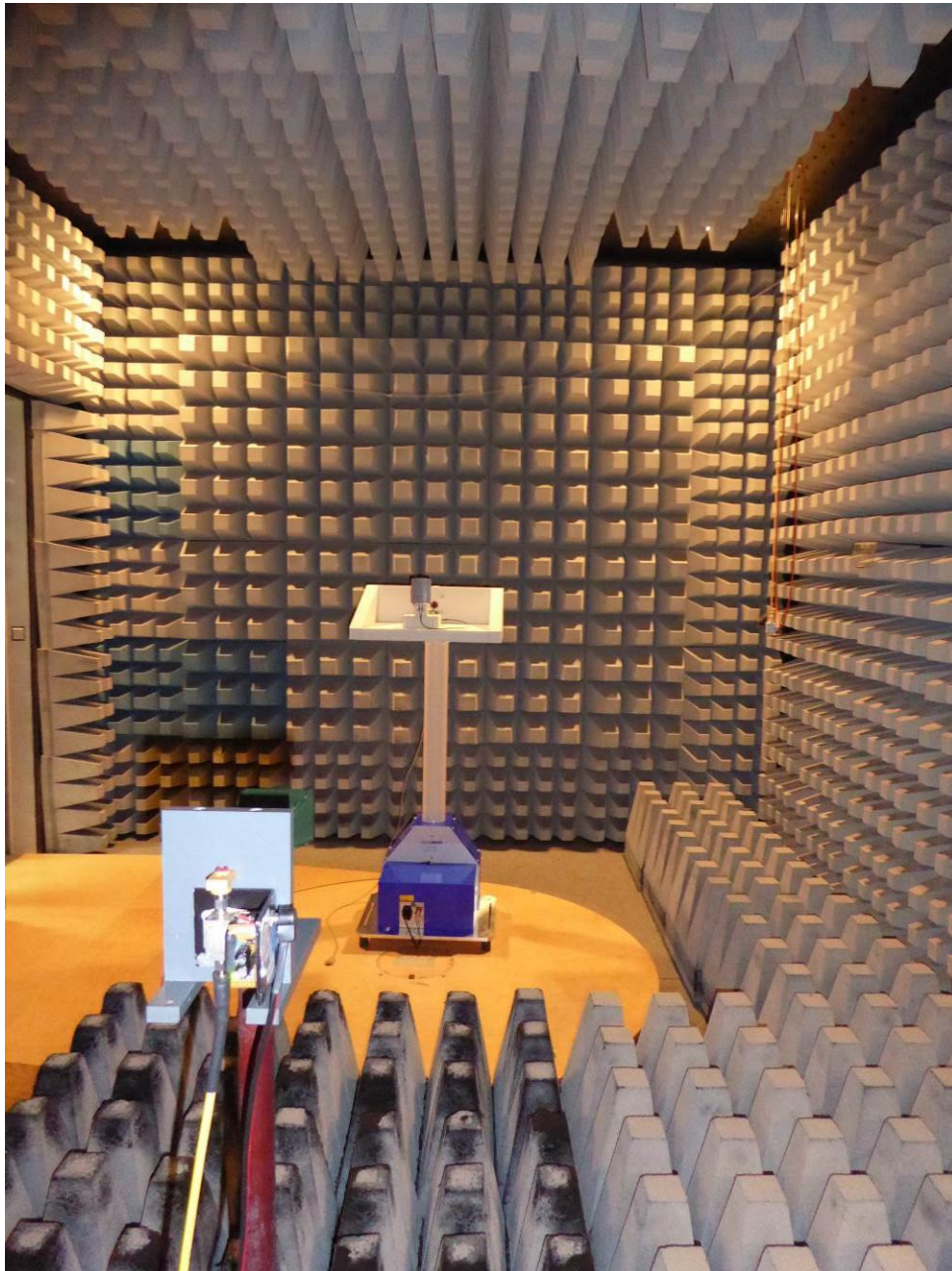
161419_12: Test setup - Radiated emission anechoic chamber
