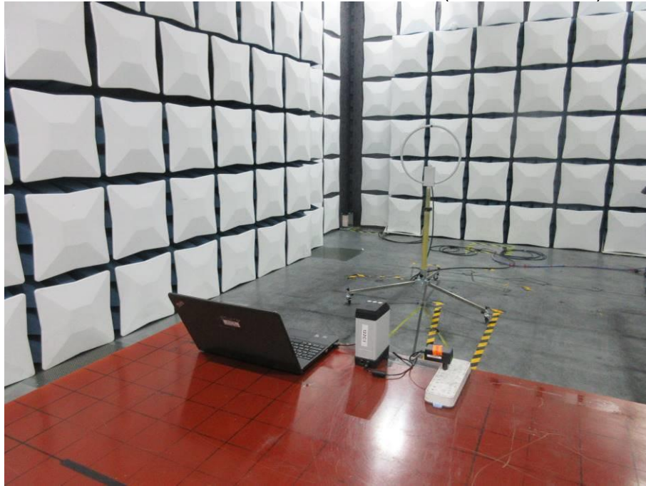
RADIATED RF MEASUREMENT SETUP (9KHz ~ 30 MHz)
