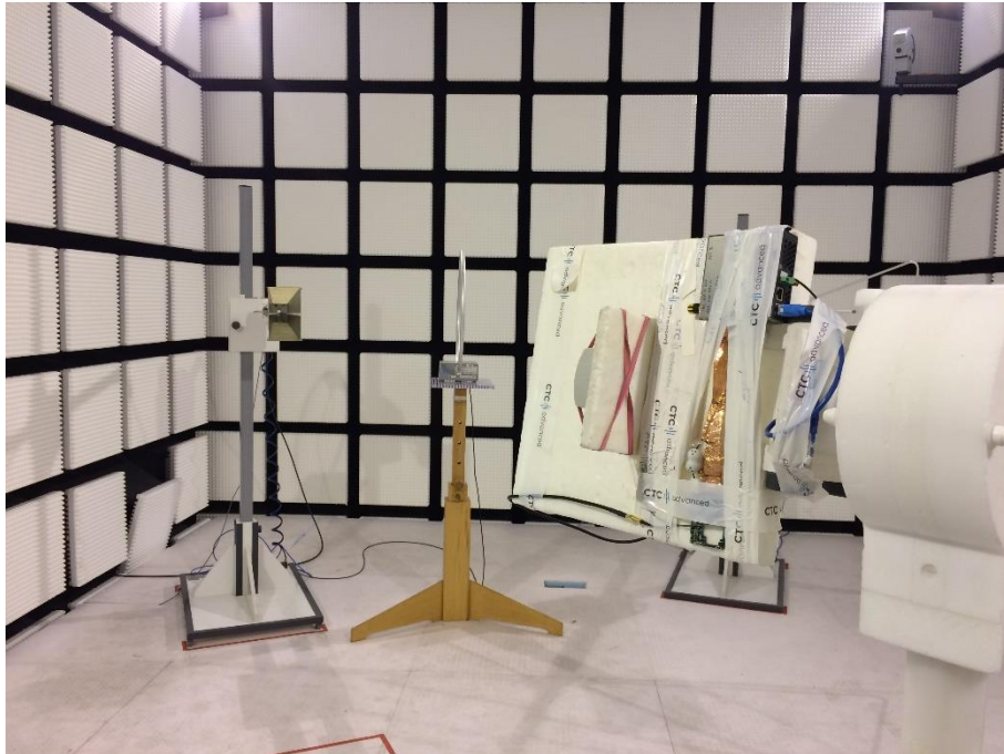
Photo 5: RSE set-up (>1GHz)
