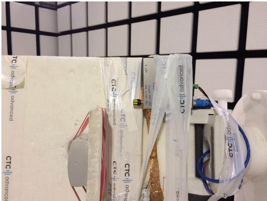
Photo 4: RSE set-up (>1GHz)
