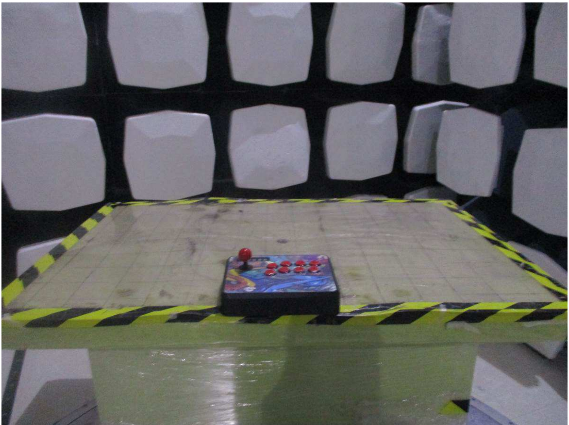
Up to 1GHz (The EUT placed at the center of the turntable)
