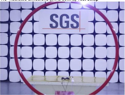
1.7 Radiated Emissions (30MHz-1GHz) Test Setup
