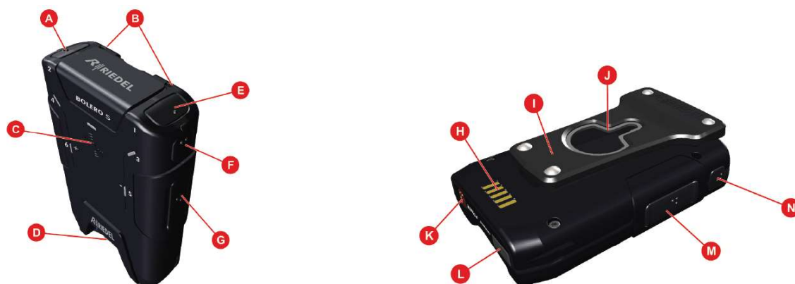
Figure 205: S-Beltpack – Operating Elements (front/top, rear/bottom)
