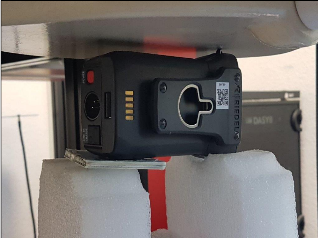
Photo 5: EUT Test Position right 5mm
