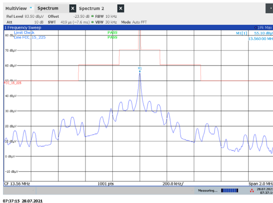
Plot 2: Spectrum mask (the limits are recalculated according to the ANSI C63.10-2013 sub clause 6.4)
