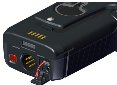
Figure 195: Pull rubber cover
