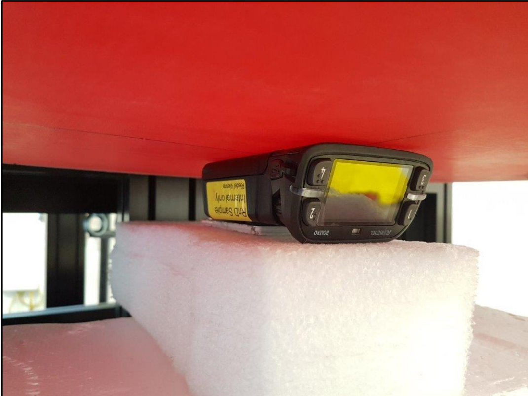
Photo 15: RFID test position - bottom side with 0mm distance
