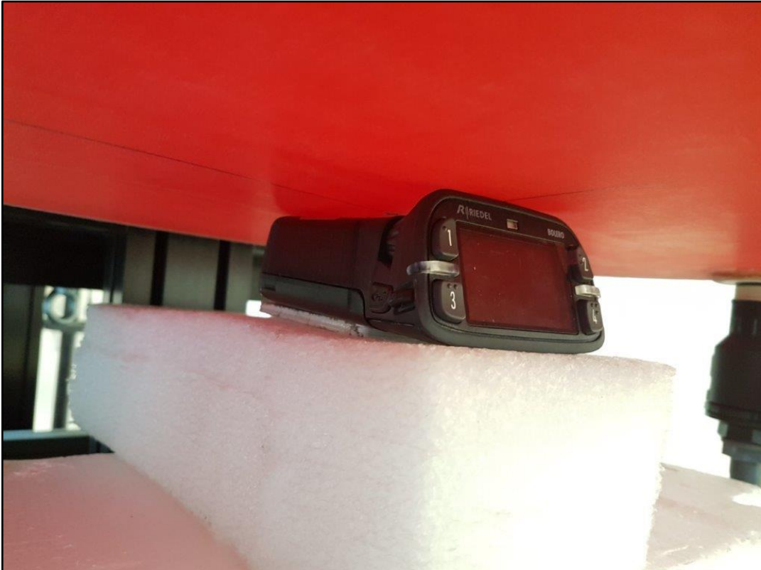
Photo 12: RFID test position – top side with 0mm distance
