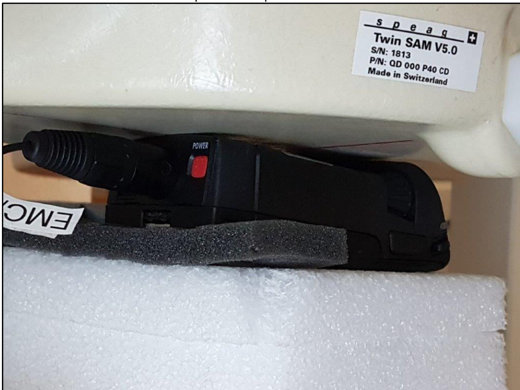
Photo 6: Test position – top side with 0mm distance
