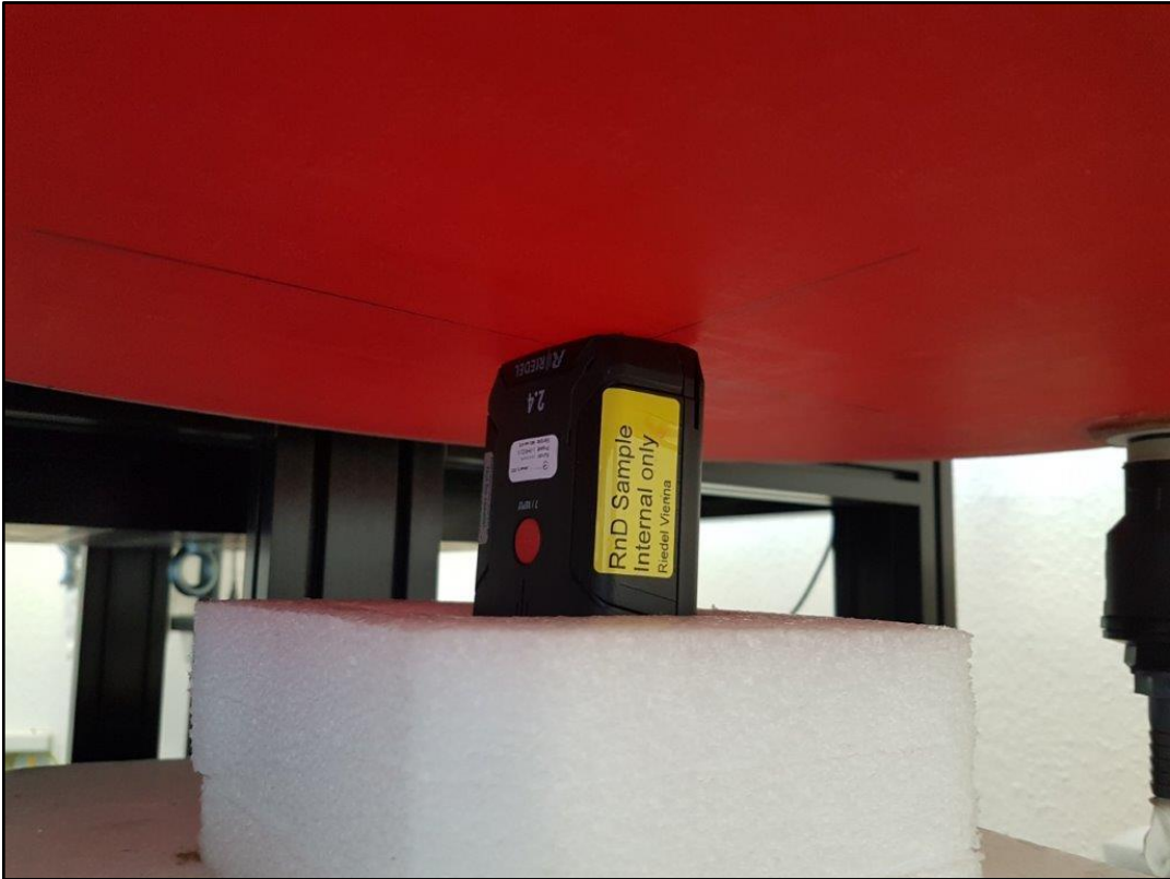
Photo 12: RFID test position – top side with 0mm distance
