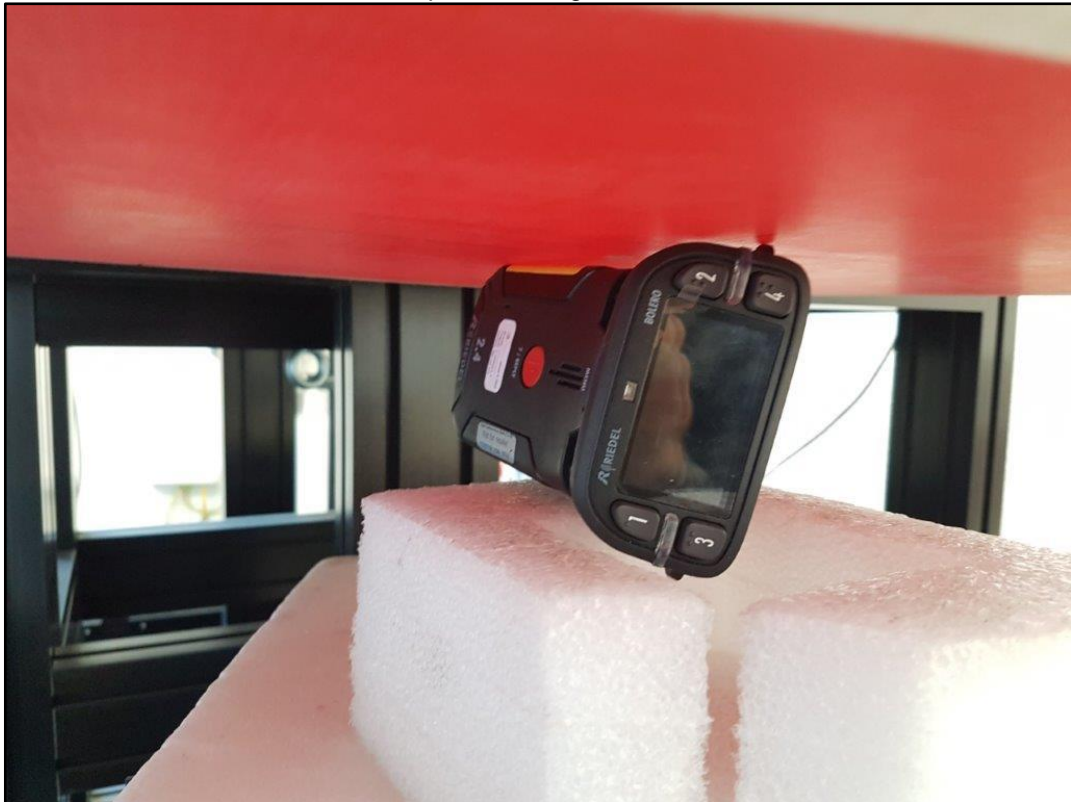
Photo 14: RFID test position - Right side with 0mm distance
