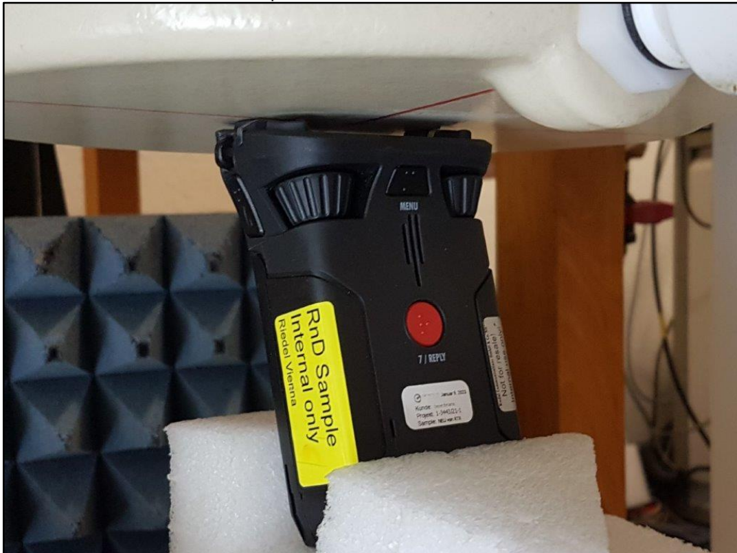
Photo 5: Test position – front side with 0mm distance
