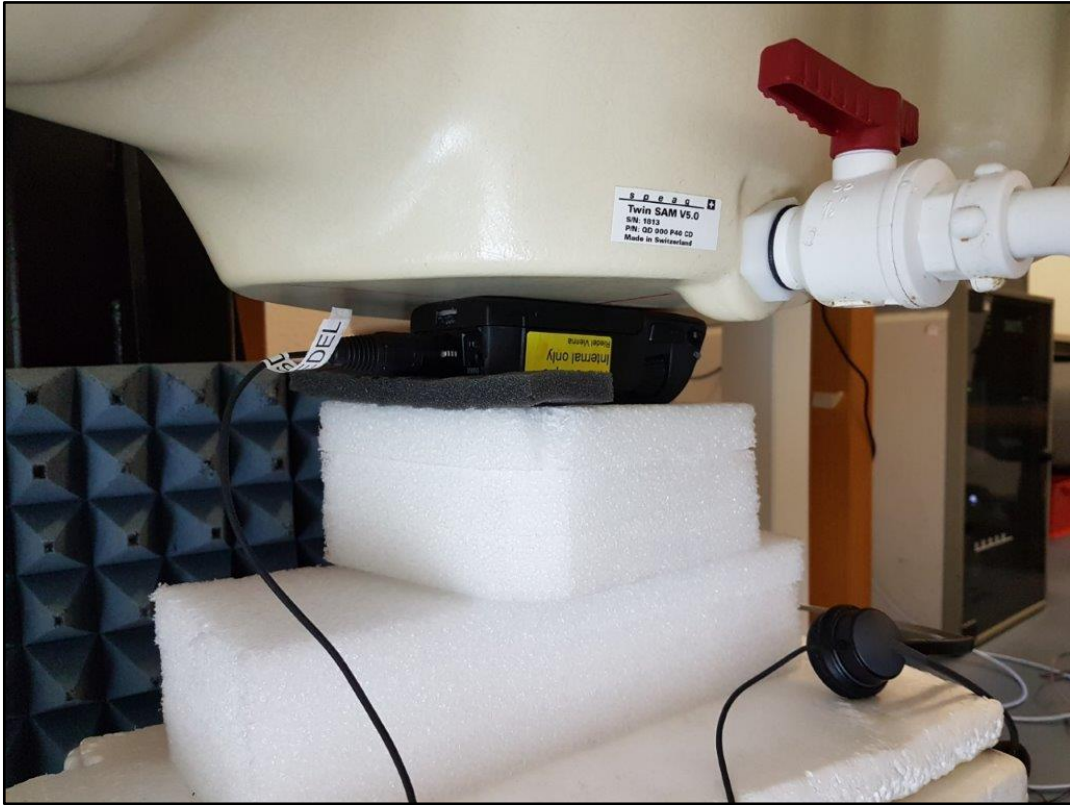
Photo 9: Test position - bottom side with 0mm distance
