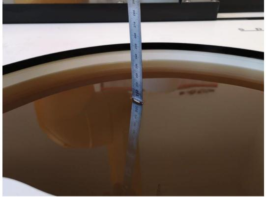
Photo 1: Liquid depth HBBL600-10000MHz Simulating Head Liquid
