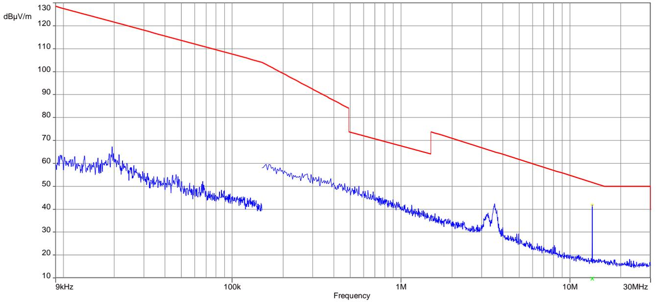
**Plot 2: Spectrum mask (the limits are recalculated according to the ANSI C63.10-2013 sub clause 6.4)**
