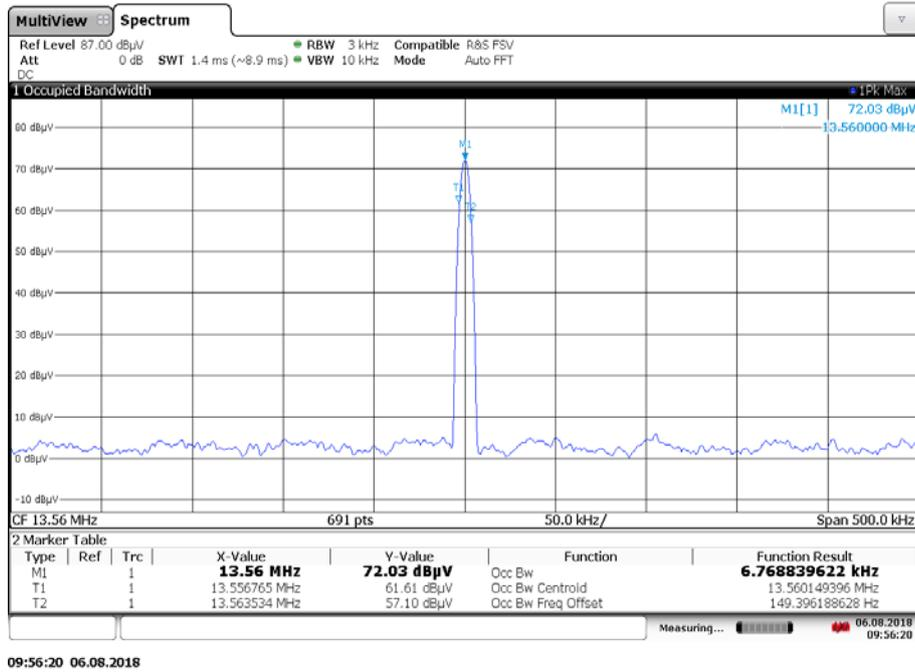
\*The signal was unmodulated carrier so there is a slight variation in the Resolution bandwidth and doesn't fall within the range of 1- 5 % of OBW
