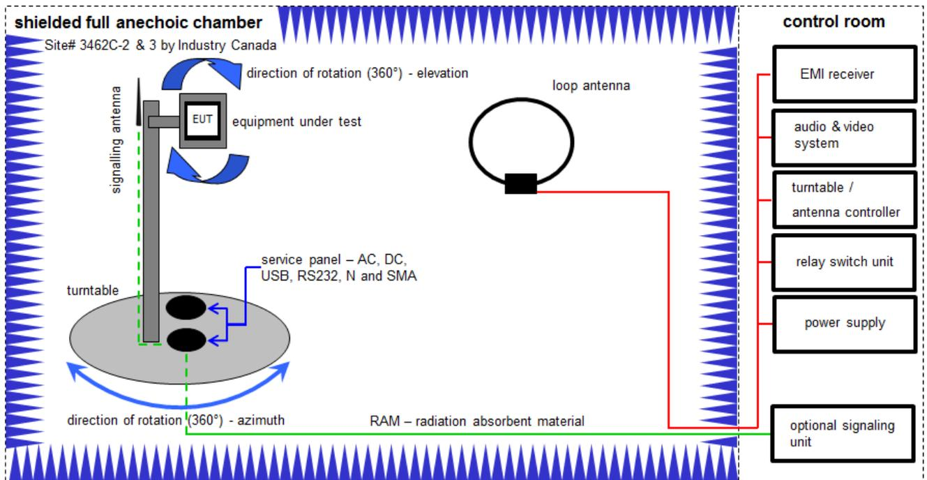
Measurement distance: loop antenna 3 meter / 1 meter
