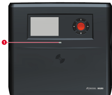
Figure 5: Antenna (Status LED positions front)
