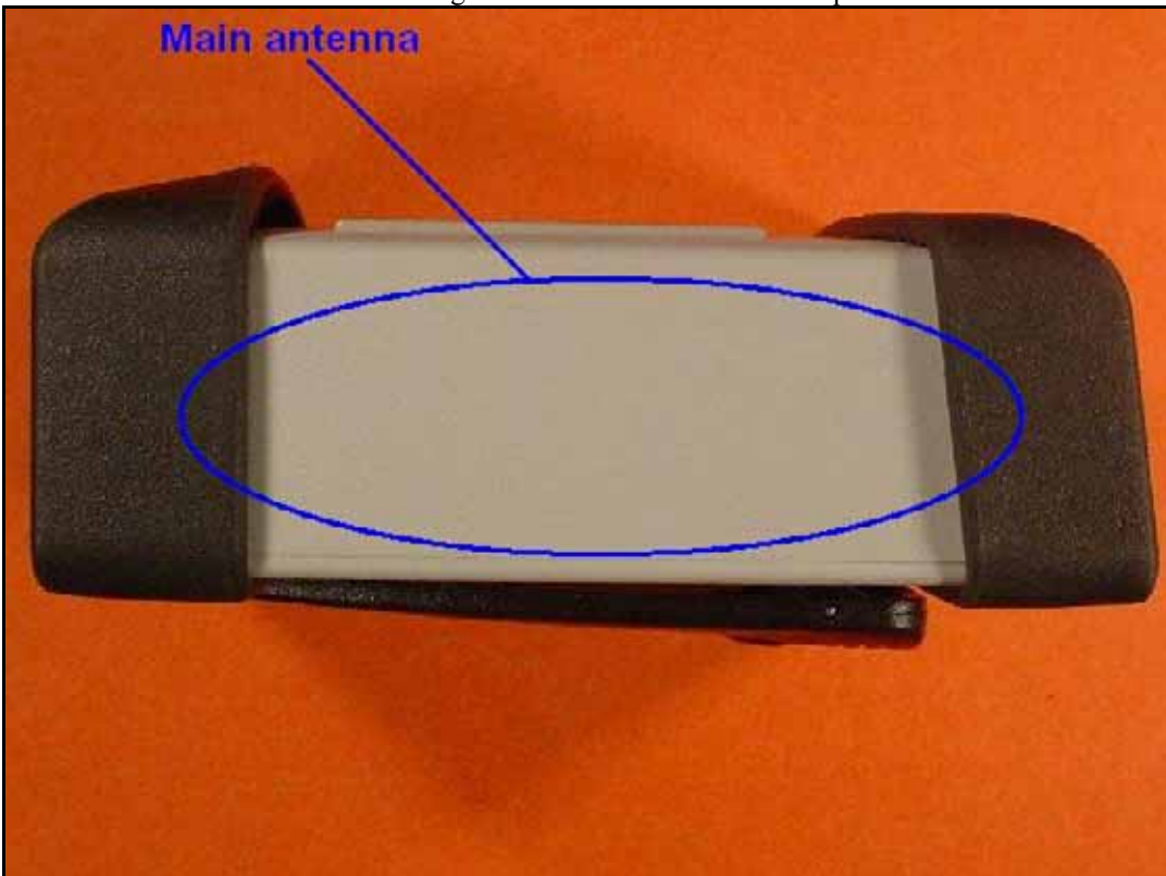
Photo 6: DUT - right hand side view with antenna position
