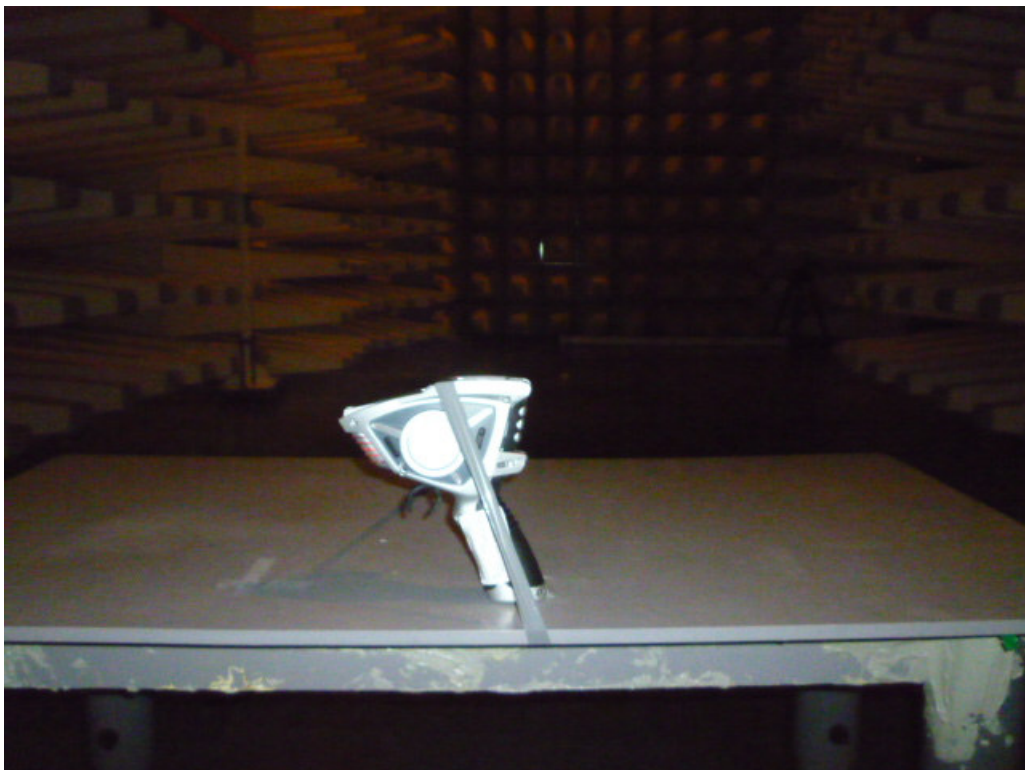
Set-up for Radiation Emission (Transceiver)
