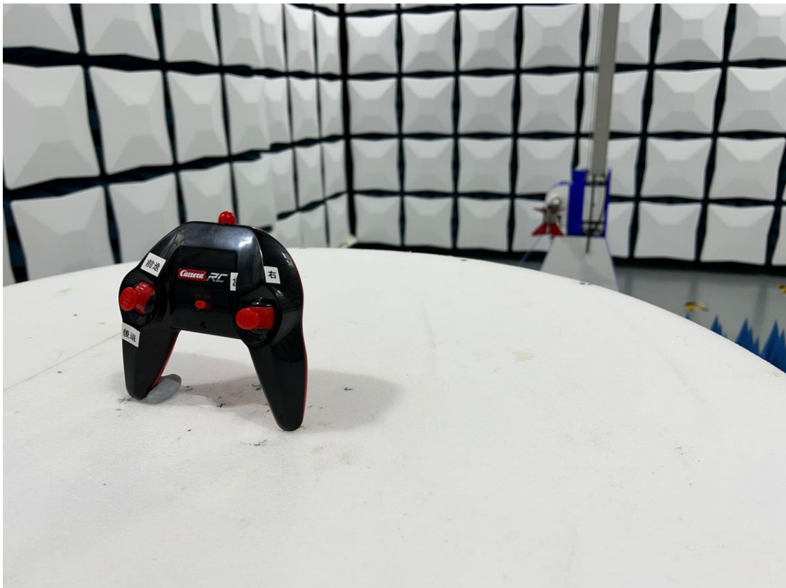
Set-up for Radiated Emission (1GHz above)
