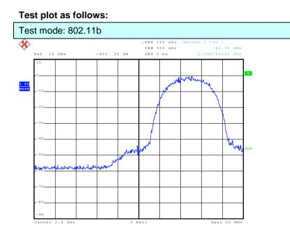
Lowest channel Test mode: 802.11b \*RBW 100 kHz Marker 1 [T1 ] \*VBW 300 kHz -60.49 dBm SWT 5 ms 2.484600000 GHz Ś Att 30 dB Ref 0 dBm 1 PK MAXH annowerherfeligeournering here mark shnalu 2.4835 GH: Span 50 MHz enter МНz
