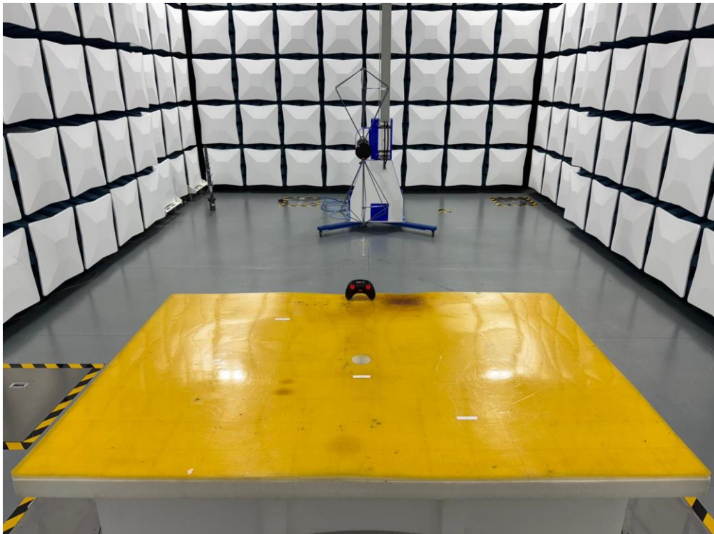
Set-up for Radiated Emission (30MHz-200MHz)
