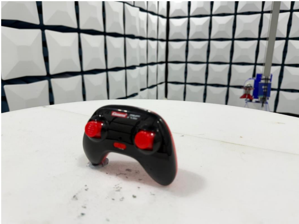
Set-up for Radiated Emission (1 GHz above)
