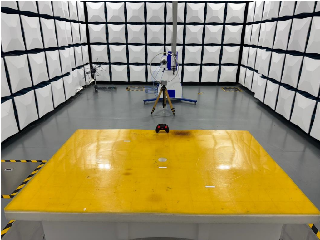
Set-up for Radiated Emission (9kHz-30MHz)
