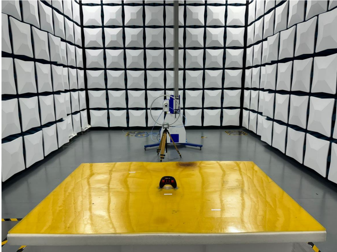
Set-up for Radiated Emission (9k-30MHz)
