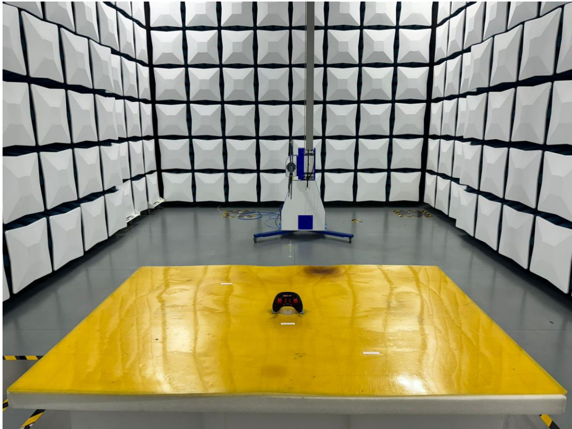
Set-up for Radiated Emission (200-1000MHz)
