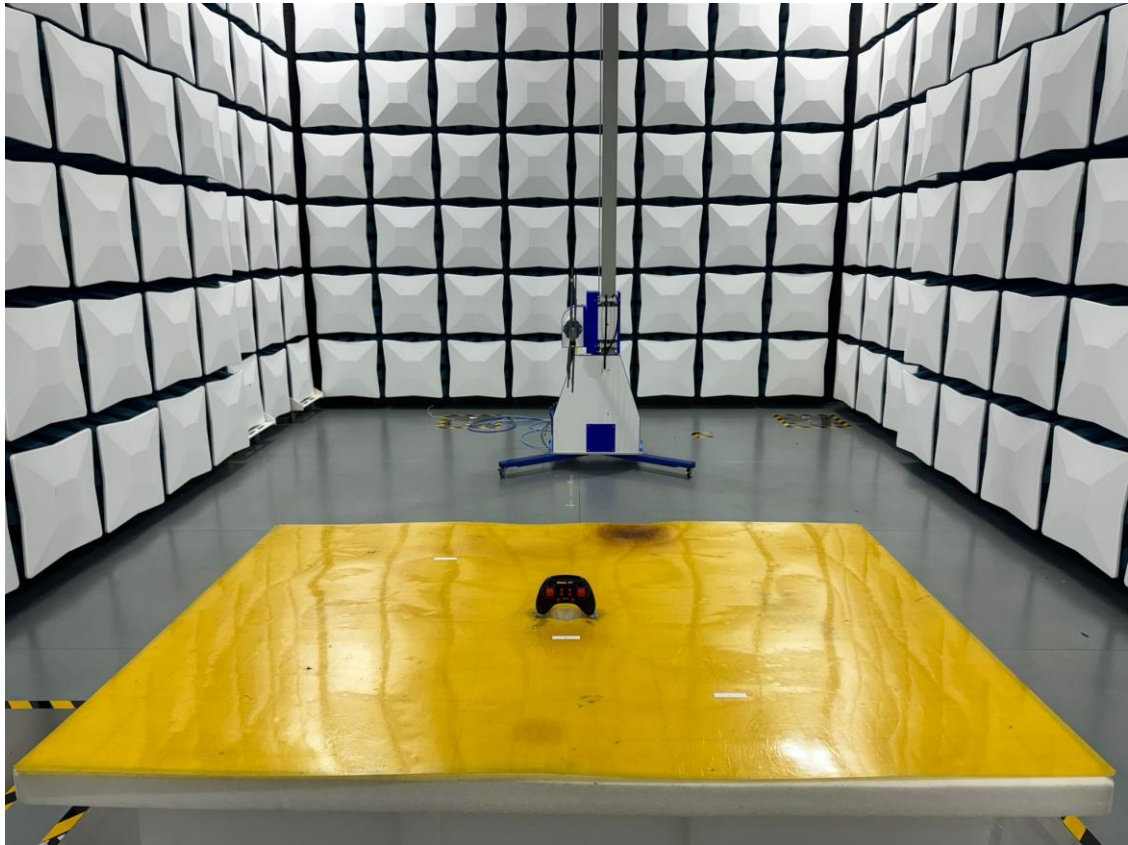
Set-up for Radiated Emission (200-1000MHz)
