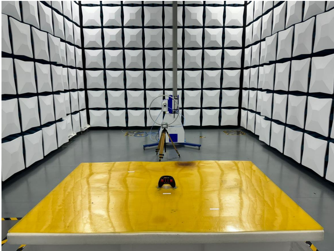
Set-up for Radiated Emission (9k-30MHz)
