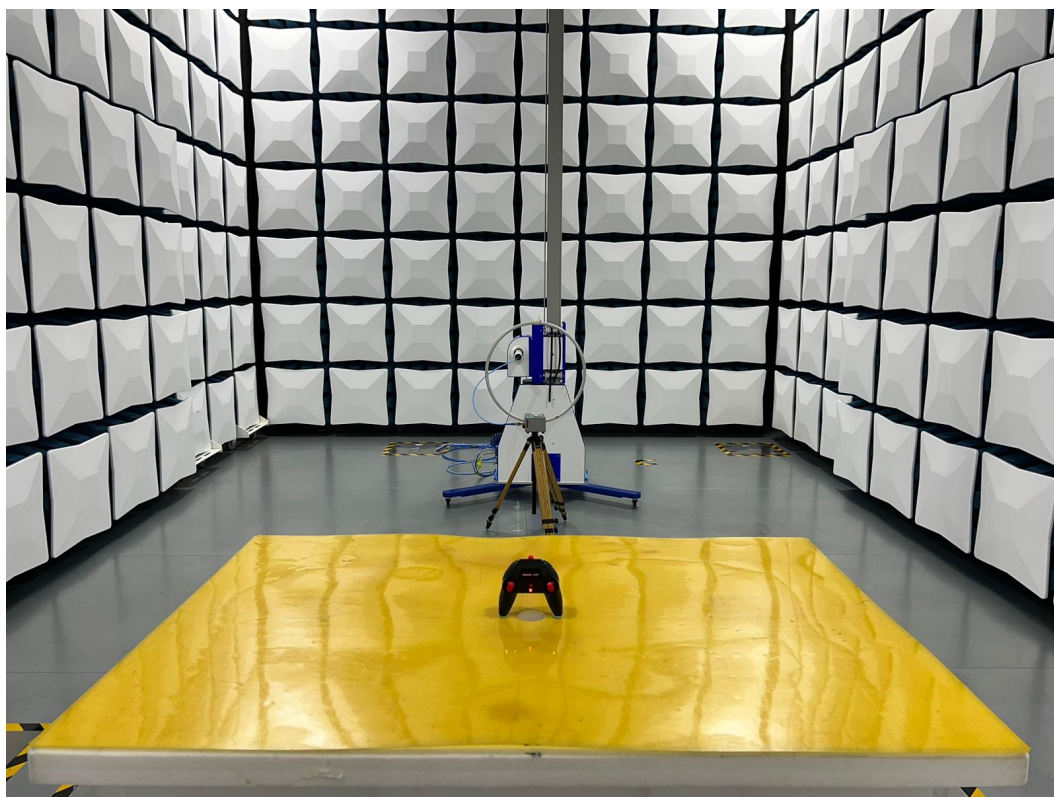
Set-up for Radiated Emission (9k-30MHz)
