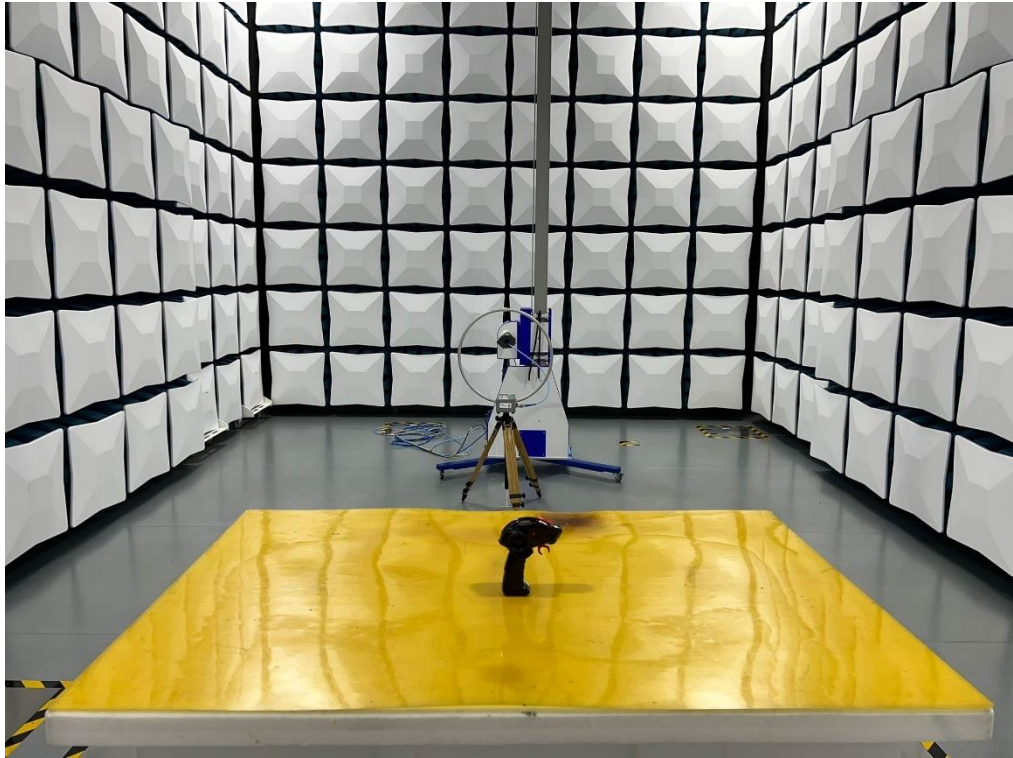
Set-up for Radiated Emission (9k-30MHz)
