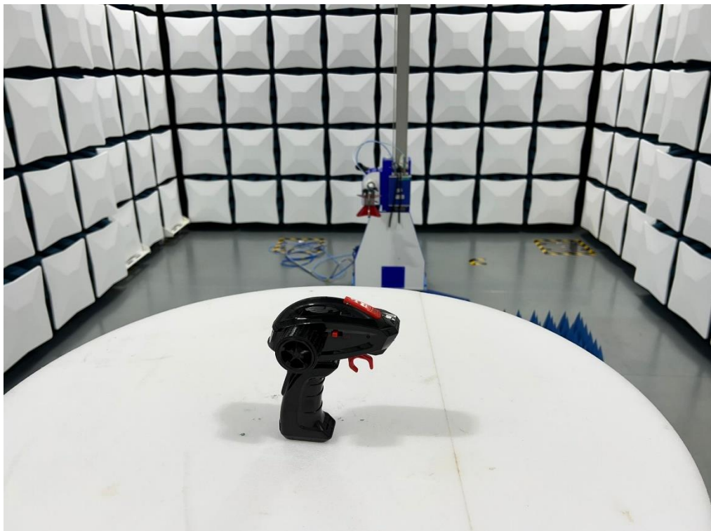
Set-up for Radiated Emission (1GHz above)
