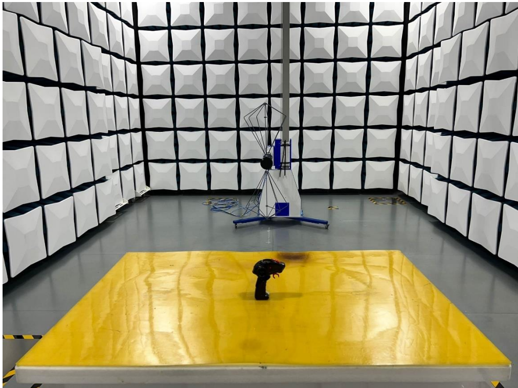
Set-up for Radiated Emission (30M-200MHz)
