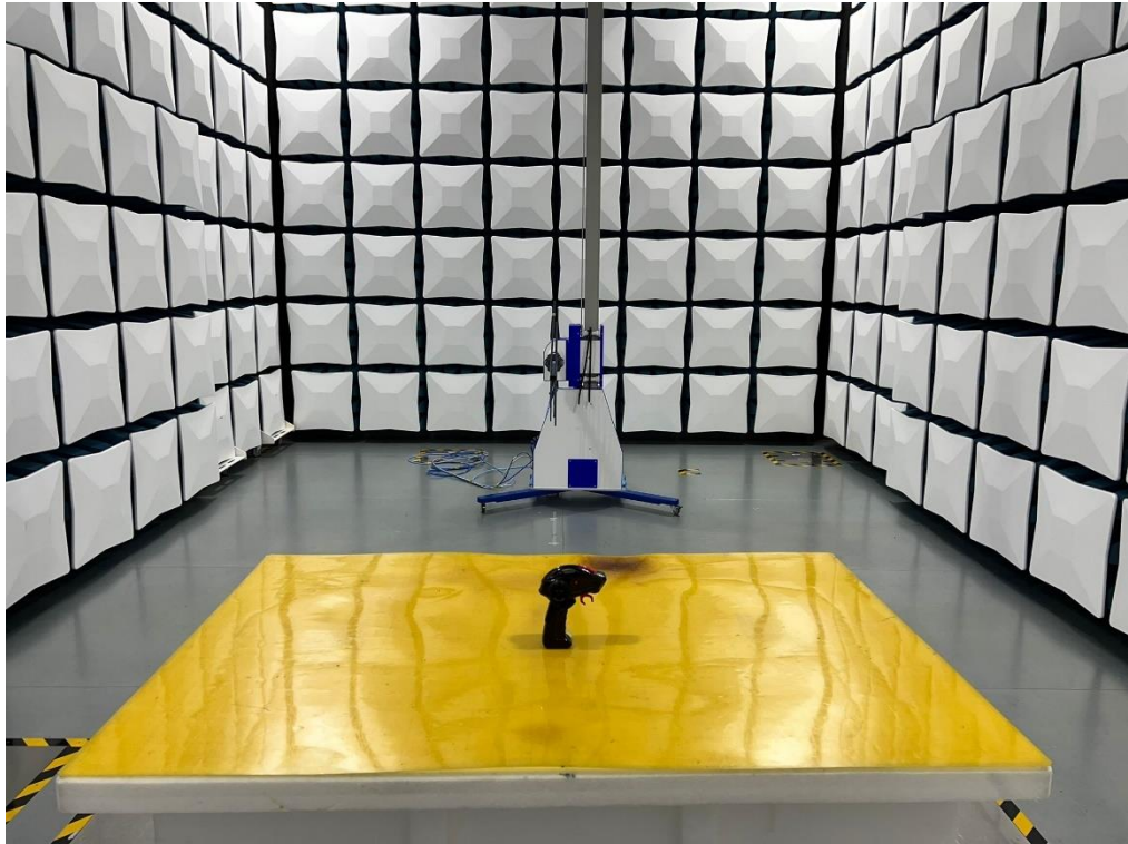
Set-up for Radiated Emission (200M-1GHz)
