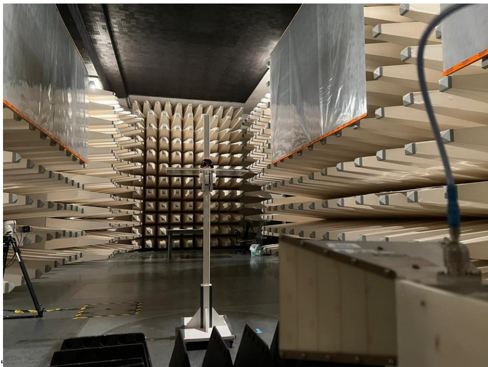
Set-up for Radiated Emission (1GHz above)
