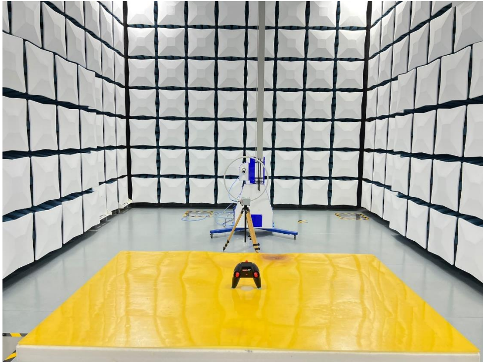
Set-up for Radiated Emission (9k-30MHz)
