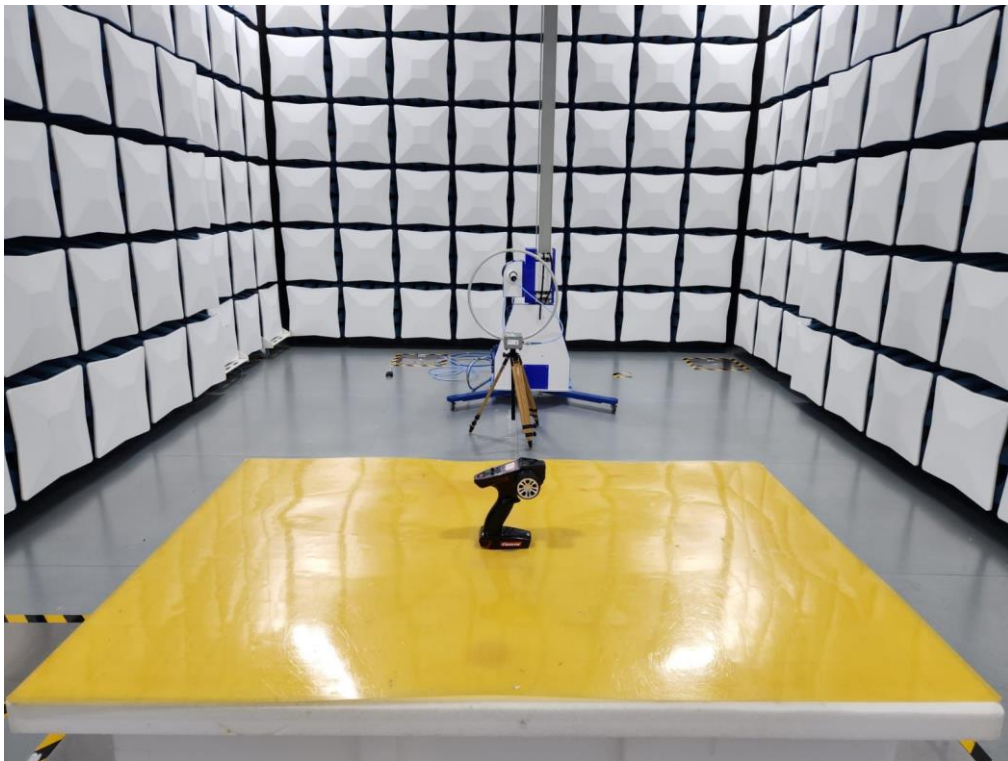
Set-up for Radiated Emission (9k-30MHz)
