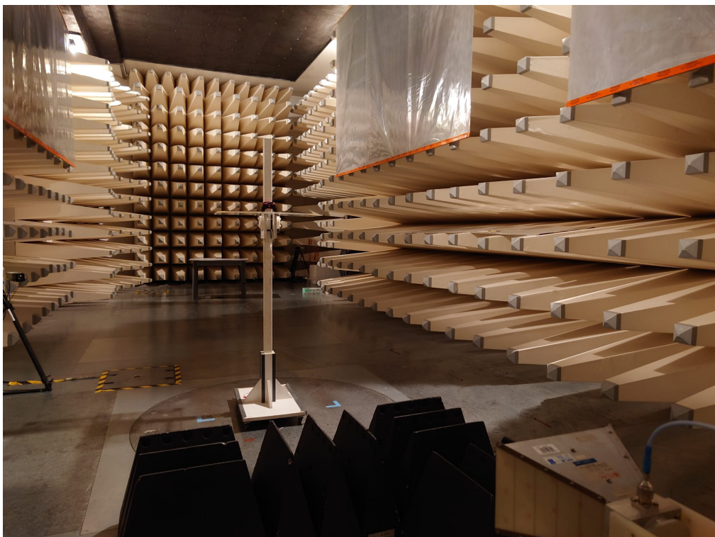
Set-up for Radiated Emission (1GHz above)
