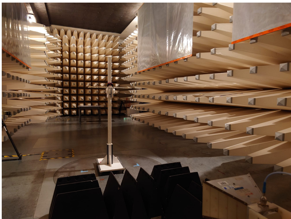
Set-up for Radiated Emission (1GHz above)
