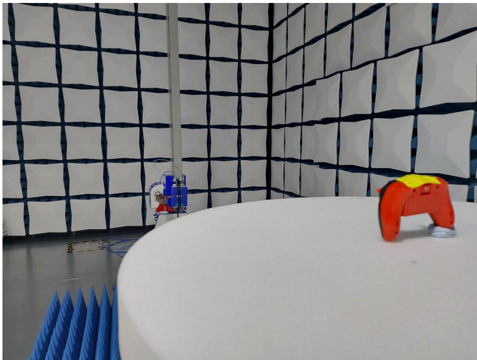
Set-up for Radiated Emission (1GHz above)
