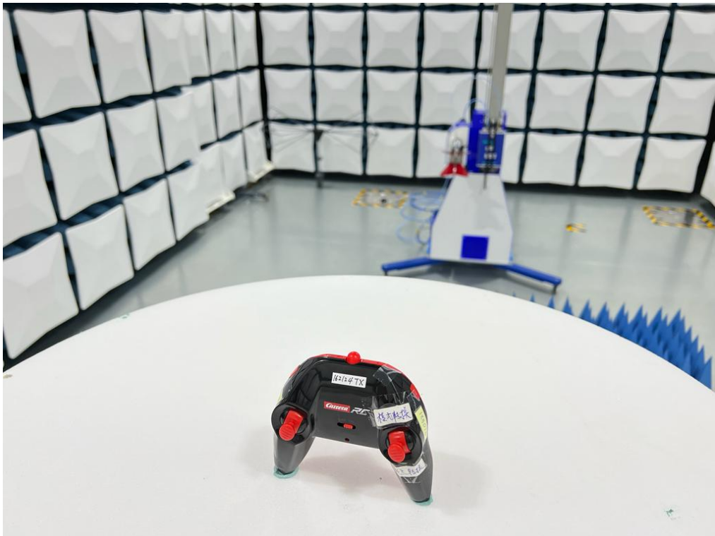
Set-up for Radiated Emission (1GHz above)
