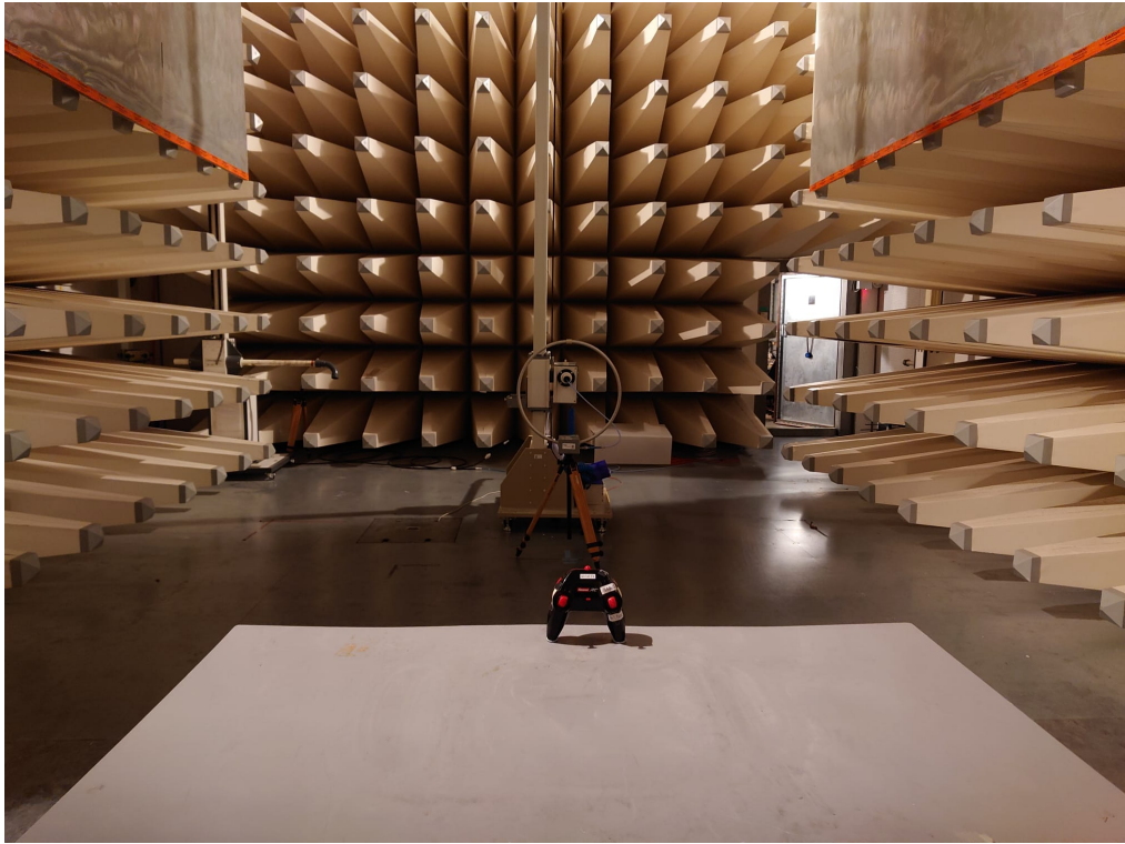
Set-up for Radiated Emission (9k-30MHz)
