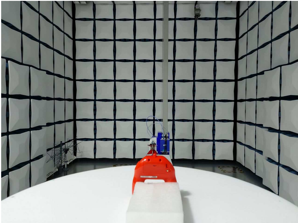
Set-up for Radiated Emission
