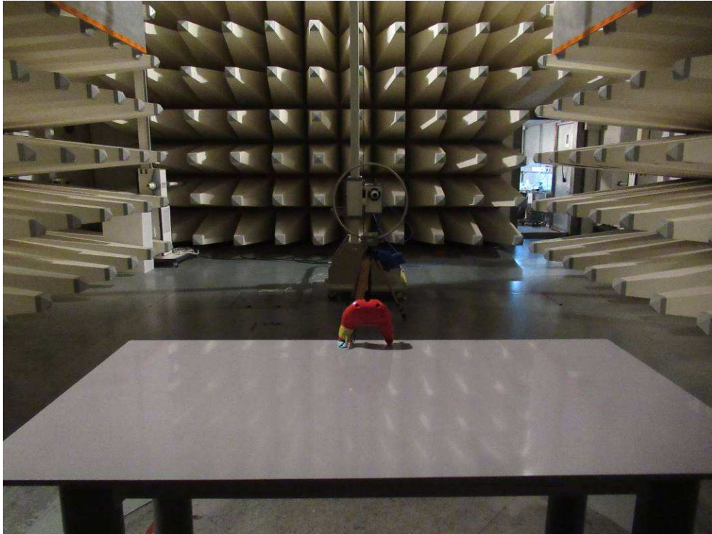
Setup for Radiated Emissions
