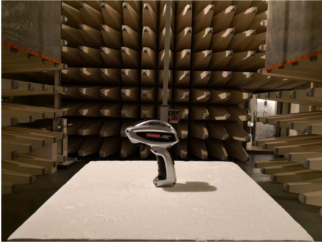
Set-up for Radiated Emission
