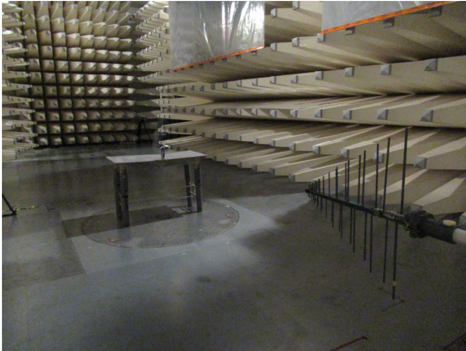
Setup for radiated emission
