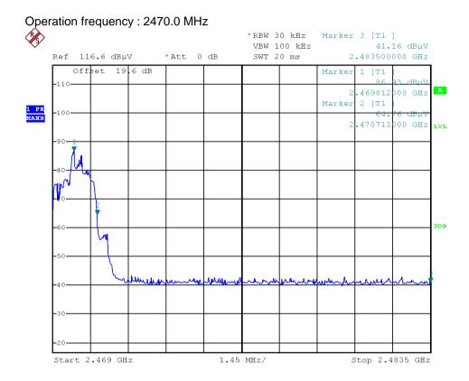
According to above plot, 20dB bandwidth falls in assigned band (2400-2483.5)MHz. It is deemed to comply with section 15.215
