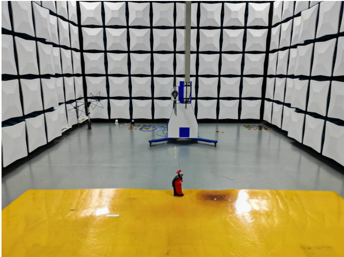
Set-up for Radiated Emission (200-1000MHz)
