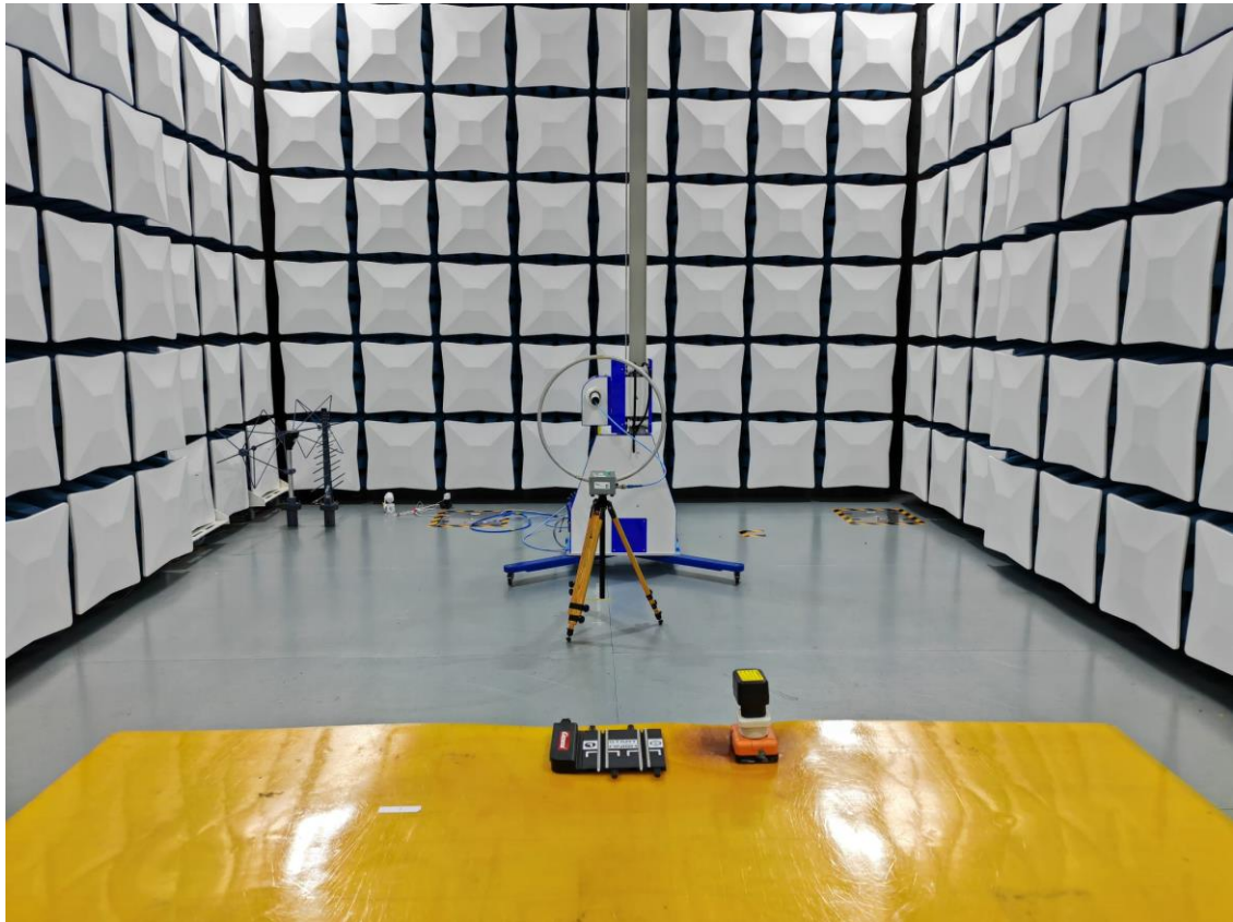
Set-up for Radiated Emission (9k-30MHz)
