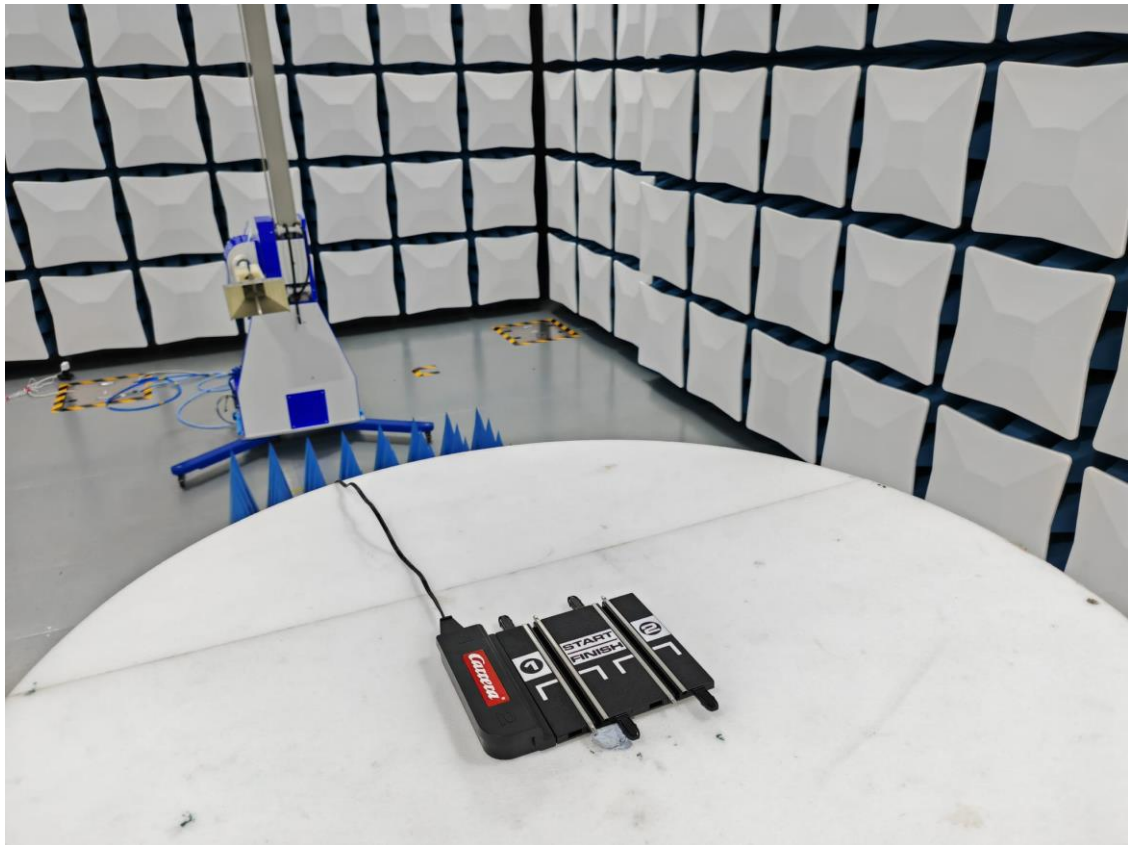
Set-up for Radiated Emission (1GHz above)
