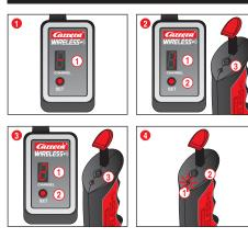
Before the speed controller can be used to control the cars, it must be "bound" to the receiver.
