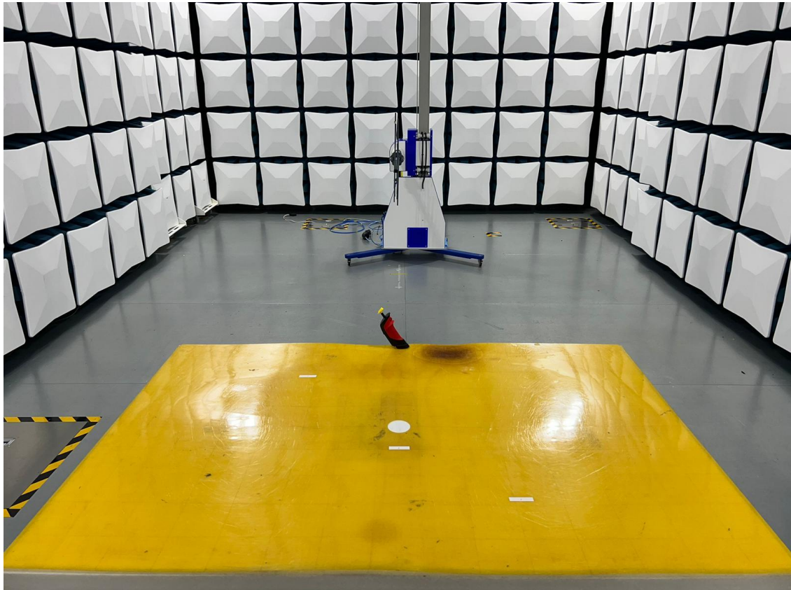
Set-up for Radiated Emission (200-1000MHz)
