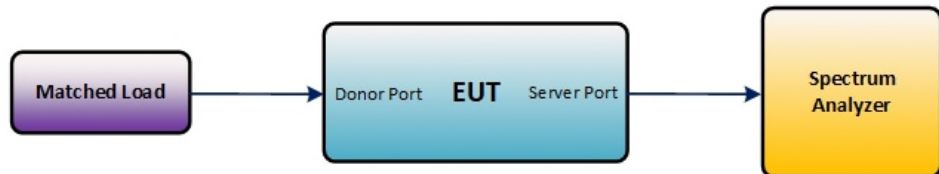
Figure 6 – Maximum downlink noise limit test configuration
