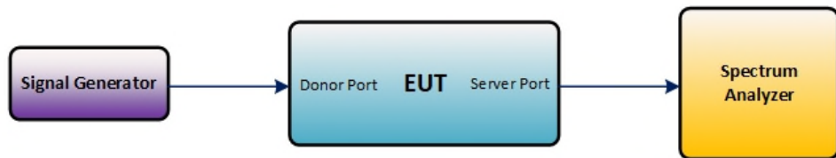
Figure 5 – Intermodulation product instrumentation test setup
