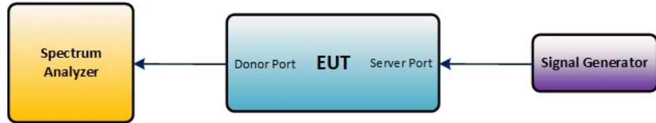
Figure 3 – Downlink test configuration in EUT test mode
