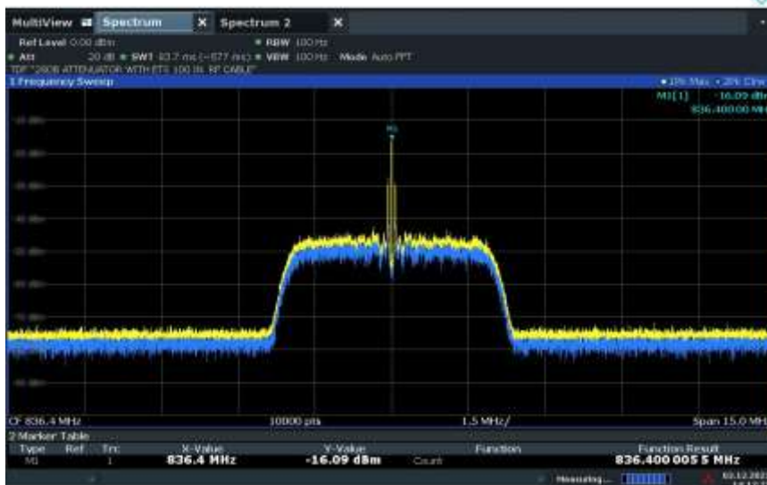
WCDMA B5 Uplink Middle Channel 120VAC @ -30°C
