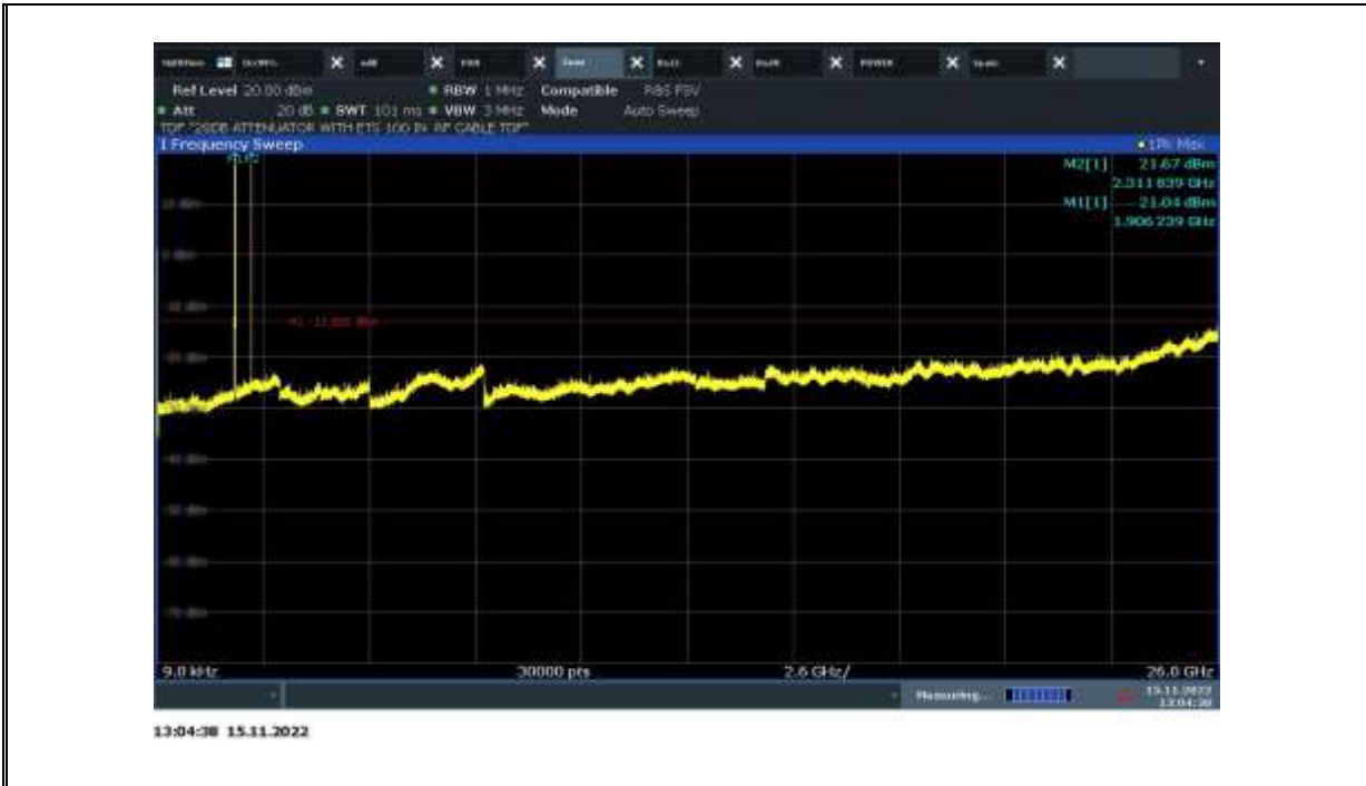
2 Bands per antenna Port 2 conducted Spurious Emissions Antenna Port 1 Uplink: WCDMA Band 5 5MHz BW Mid Ch & LTE Band 12 10MHz BW Low Ch
