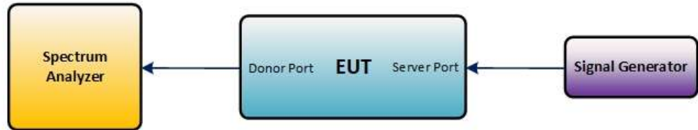
Figure 3 – Downlink test configuration in EUT test mode
