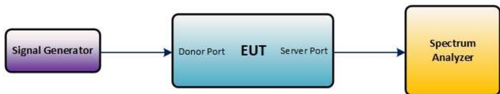
Figure 5 – Intermodulation product instrumentation test setup
