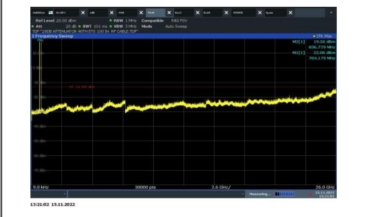
2 Bands per antenna Port 2 conducted Spurious Emissions Antenna Port 1 Uplink: WCDMA Band 5 5MHz BW Mid Ch & LTE Band 30 5MHz BW High Ch
