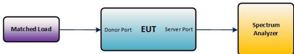
Figure 6 – Maximum downlink noise limit test configuration
