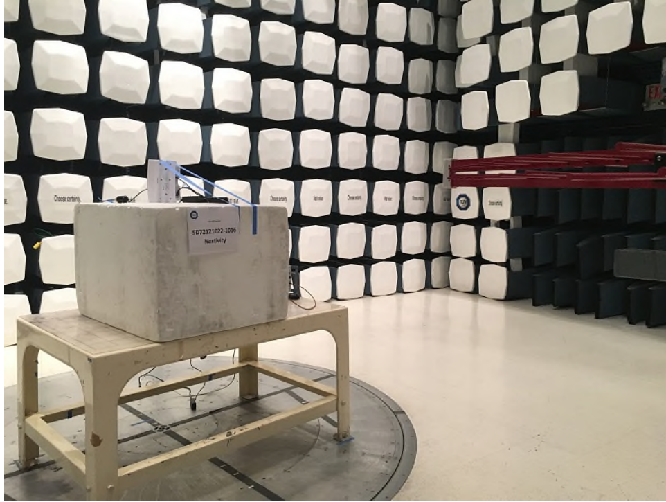
NU Radiated Emissions Below 1GHz Front
