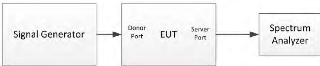
Figure 3: Downlink Test Configuration in Test Mode
