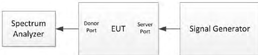
Figure 2: Uplink Test Configuration in Test Mode
