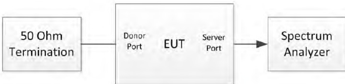
Figure 5: Maximum downlink noise limit test configuration
