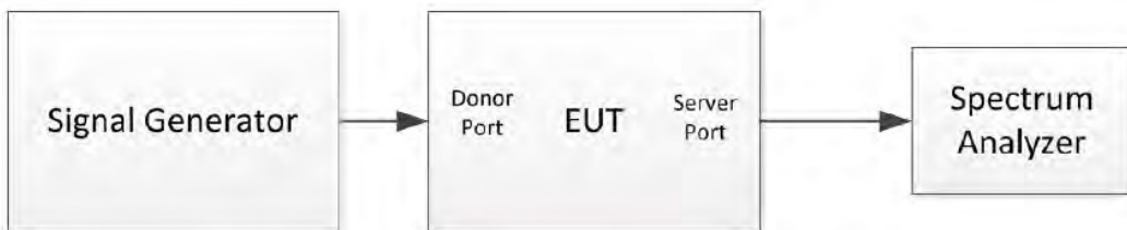
Figure 3: Downlink Test Configuration in Test Mode
