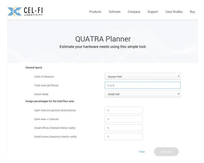
The QPT algorithms are based on ever-evolving IEEE 802.16 propagation models, and will provide a very good estimate in most cases. Once on site, it's always good to measure actual values to ensure best performance, and for any solution adjustments.
