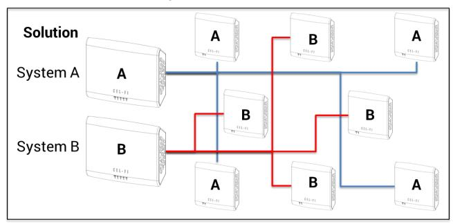
A QUATRA system is comprised of a Network Unit (NU) and one to four Coverage Units (CU). An NU and CU are paired; they must be of the same model, and band configuration. Multiple QUATRA systems can be installed together to form a larger solution. Systems can be attached to a specific site in WAVE, and managed accordingly. A site represents a physical location, in WAVE.
