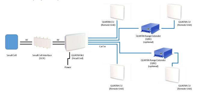
A Supercell is comprised of a Cel-Fi QUATRA 1000 system connected to a small cell. Multiple Cel-Fi QUATRA 1000 systems can be connected to a single small cell, or multiple small cells, to form a coordinated Supercell that extends coverage for large venues. A Supercell with multiple Cel-Fi QUATRA 1000 coverage units (CUs) is more efficient than multiple small cells, and the CUs of a Cel-Fi QUATRA 1000 system connected to a Supercell do not interfere with one another.
