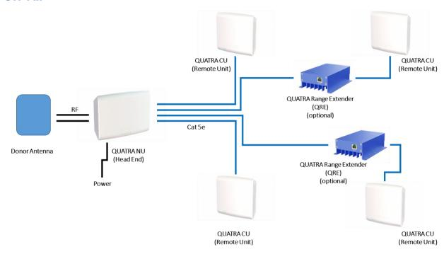
Cel-Fi QUATRA can be installed off-air to provide high-quality in-building wireless connectivity by using the existing cellular network. Off-air installations comprised of an NU and up to four (4) distributed CUs dynamically networked into a single system to provide high-quality in-building wireless connectivity.
