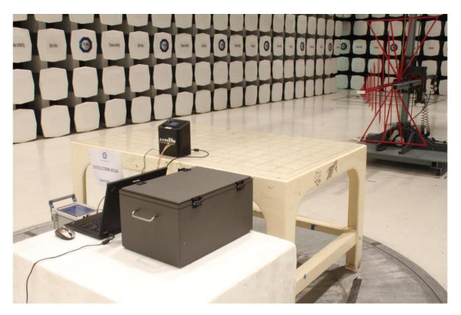
Radiated Emissions Test Setup (below 1GHz)
