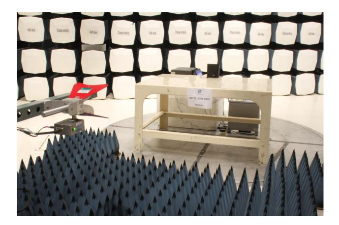
Radiated Emissions Test Setup (above 1GHz)
