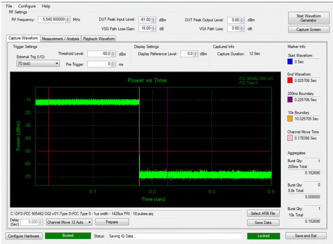
5540 MHz Zoomed In Overall Power vs Time Display, showing Channel Move Time (Pink), end of Radar Burst (Red) and the 200 ms boundary (Purple)
