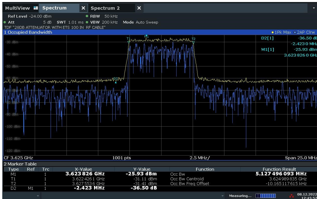
99% OBW Input Signal Profile (5MHz)
