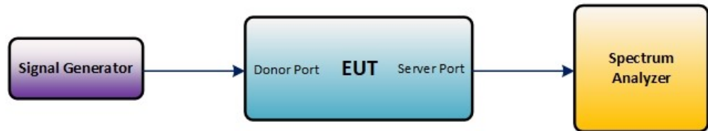
Figure 3 – Downlink test configuration in EUT test mode
