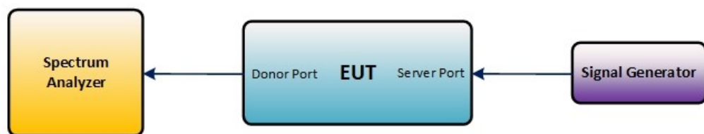
Figure 2 – Uplink test configuration in EUT test mode
