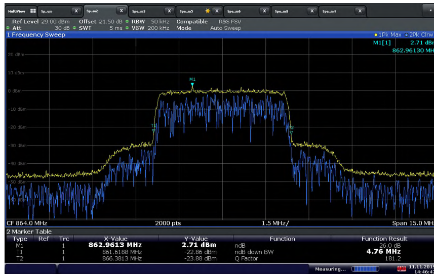
LTE Band 26 (859 – 869 MHz) Downlink 5MHz BW / Middle Channel 864 MHz / 26dB BW
